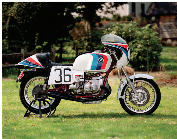
By 1978, Japanese machines should've ruled in AMA Superbike. But Udo Gietl's ingenuity ensured they didn't. His 1978 R90S featured a homemade mechanical front-brake anti-dive system. Photo courtesy Udo Gietl.
